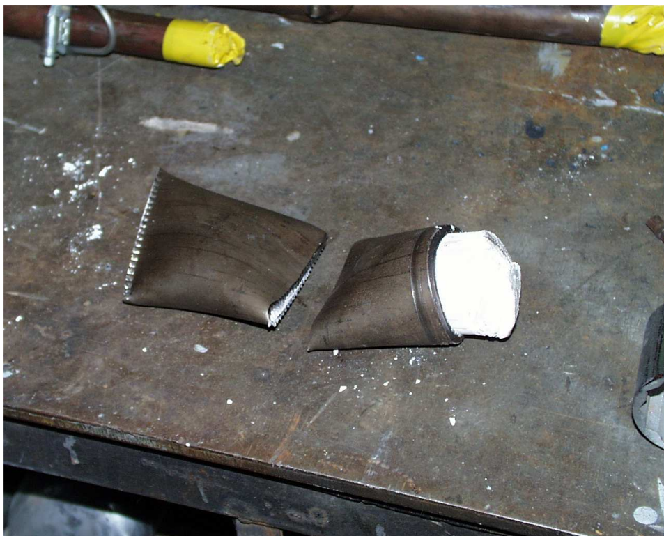
Figure 12 : Tubes full of sodium being cut with hydraulic shears
