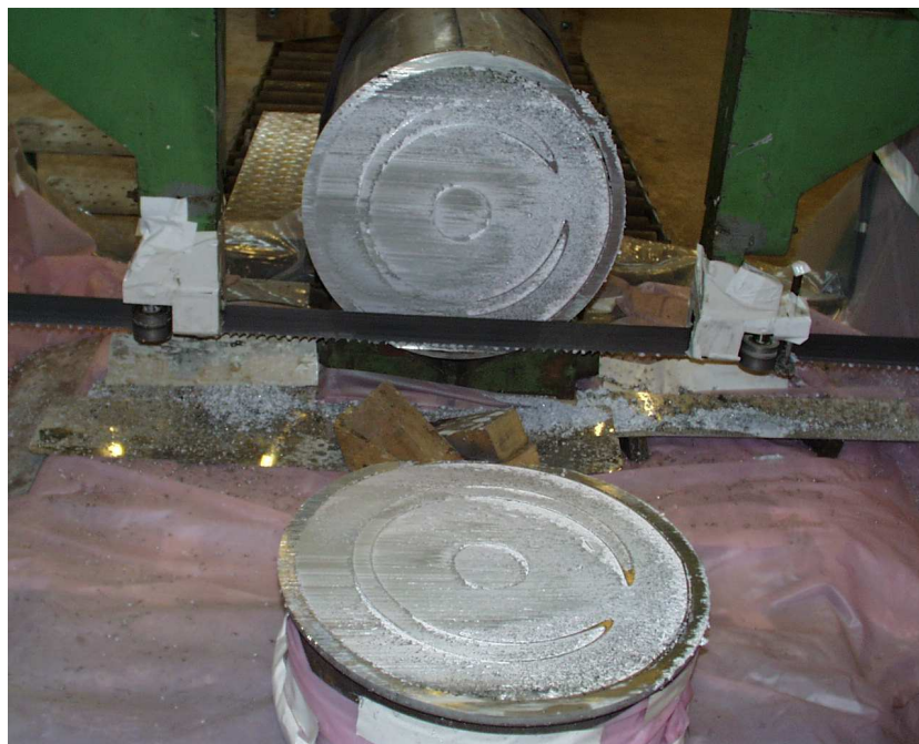
Figure 9 : Slice of cold trap full of sodium cut with a band saw
