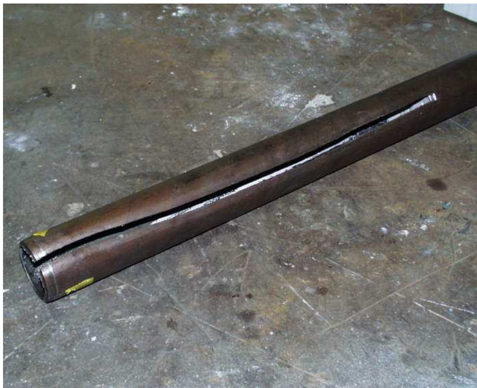
Figure 11 : Pipe with residual sodium inside being cut in its length by a nibbling machine
